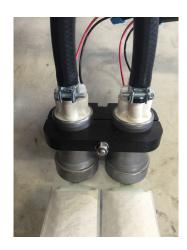
Step 15: This is what the assembled pumps and hat should look like. The hose connecting to the underside of the hat should be tightened in the position depicted below (green arrow), this is important so the hose does not jam the fuel level sender arm during operation.
