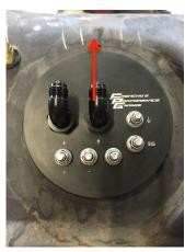
Step 21: Install the lock ring to hold the hat in place.
