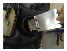
Step 8: Slide the base plate into the factory holder until it clips into place.
