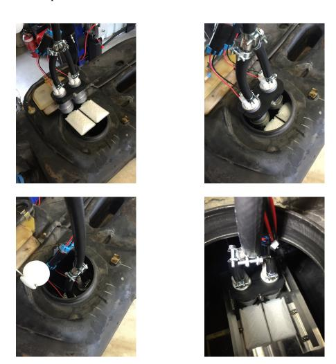
Step 17: Install the second half of the clamp and secure with the three washers and locknuts. Do not over tighten the locknuts, 6-8N.m of torque should be sufficient.
