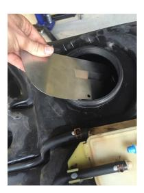
Step 11: Once the baffle is inside the tank, place it over the bolts in the base plate by squeezing the baffle together and sliding it over the bolts one side at a time.
