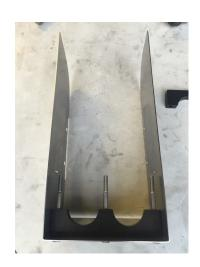
Step 10: Insert the baffle as per the pictures below:
