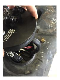
Step 20: Apply a small amount of soap on the outside of the seal to help the seal push in. Ensure the seal is engaged properly and apply downwards force to clip the hat into place in the tank. The center bulkhead (fuel supply) should line up with the notch on the fuel tank
